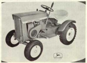
Both and 70 and 100 CADET tractors have positive gear drive--with NO BELTS--and the transmission-final drive is the same one which is used in the "World Famous" CUB.
