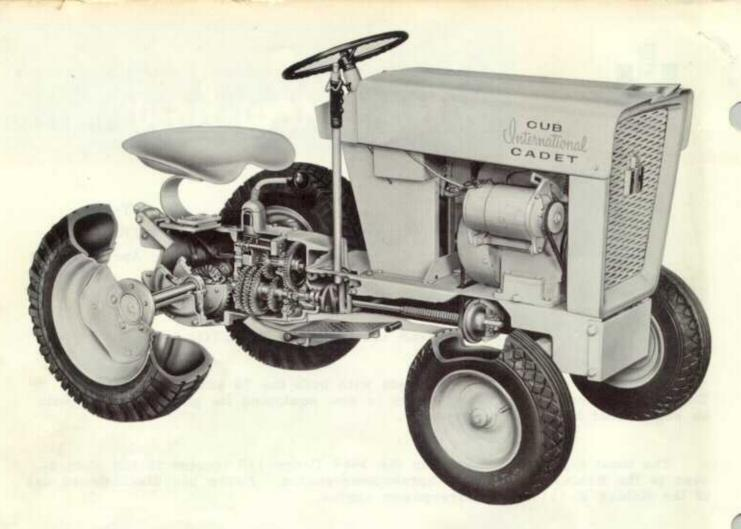
The transmission-final drive of the 70 and 100 Cub Cadet is the same one that is used in the Cub Tractor.
