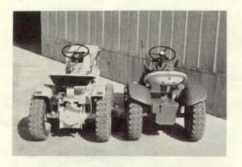
From the engine to the rear wheels there's a direct, positive transmission of power through shafts and gears. Unlike the Deere 110 and the other garden tractors, there are no power transmission belts to wear, stretch, maintain, or replace.
