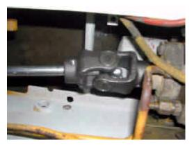
Install the U-joint kit (using one of the special pins you've made) onto the transaxle. Point the grease-fitting towards the REAR! It'll slide on to 'perfect' depth, then insert a pin through the threaded-end, line it up to the hydrostat input shaft's crosspin hole, push it through (it should be rather snug, mebbie even requiring a few taps from a light hammer), start the threads, and run it home with just a hint of end-torque.
