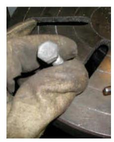
So now we employ the junk-box. First, I found a bolt which threaded into the yoke properly. This one is a Grade 5 bolt... (I don't recommend you trying this stunt with a Grade 8, unless you've got lots of sharp drill-bits that you'd like to torture). I quick chuck-it in the drill and scrub the top of the head with the 4" disk grinder to take the markings off and leave a smooth surface
