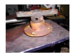
First, I started with a stock, but seriously-worn coupler. Notice how the drive-groove is waller'd out? This much slop will cause enough driveline shock to break the drive pin right off... even if it's not a bit worn.
