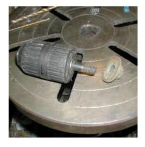
So now I'll mount this chuck to my drill-press table, with jaws facing up, and tighten it down good. Then I put a drill bit in the table-mounted chuck, facing UP. I swing the table to line up the two chucks, plunge the press chuck 'till it fits over the drill bit, and temporarily tighten the top chuck over the sharp-end of the drill bit. Then I tighten down the table adjustments... so now I know the two chucks are more-less perfectly centered.
