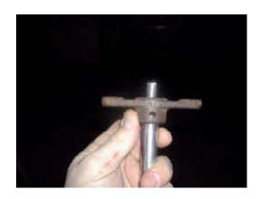
My first thought was to just make another steel plate, and drill it with three holes, then weld it onto my new shaft like the original, but decided that the reason why the factory shaft wasn't running true, was because the welding process pulled it out-of-square. Instead, I found that I had an extra rag-joint receptacle. I slipped it over the turned end...
