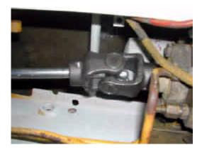
Notice- the shaft is fully bottomed against the U-joint's X-piece, but the front is well-clear of the rag joint-Plenty of room to install/remove the shaft. Notice- the U-joint's grease fitting is on the AFT side of the Xpiece- this allows lots of space for the shaft to retract for launch-pin clearance.
