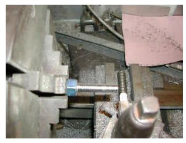
Cut off all the exposed threads... and turn it down to 0.250". I use a curved-point 'finishing' tool in the lathe- they do a nice job without yanking the workpiece out... mind you, my lathe is geriatric, so I have to do some pretty unprofessional things to get decent results. An alternative to a lathe-tool, one could use a file, or a grinder... whatever you've got will probably work with enough patience.
