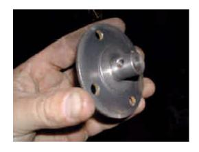
Next, I fitted the whole works together, and pressed a Spi-Rol pin into the rag-joint yoke...
