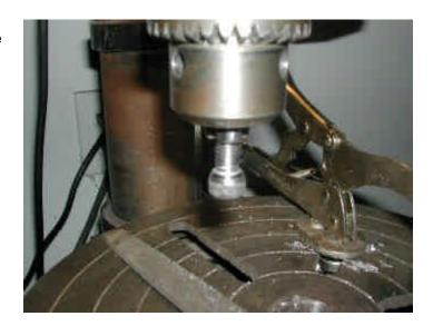
...and while I'm at it, I wipe off the casting mark along the yoke's edge, as it fouls the bolt a little, too... and the end result looks like:
